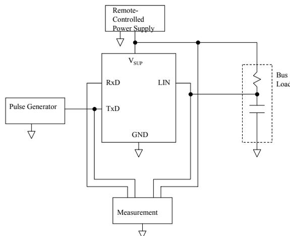
FIGURE 30—NORMAL BATTERY VOLTAGE OPERATING RANGE WITH TxD/RxD ACCESSIBLE TEST SETUP
