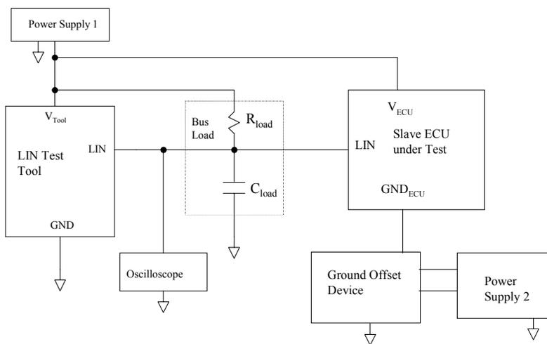
FIGURE 18—SLAVE NODE  $V_{ii}$  LEVEL MEASUREMENT TEST SETUP
