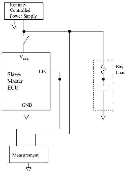
**FIGURE 26—ECU POWER LOSS LEAKAGE CURRENT MEASUREMENT TEST SETUP**
