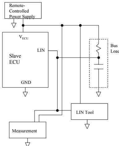
**FIGURE 31—NORMAL BATTERY VOLTAGE OPERATING RANGE WITH TxD/RxD NOT ACCESSIBLE TEST SETUP**
