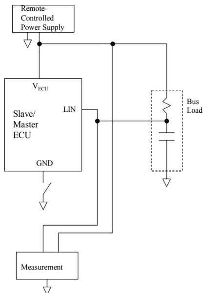
FIGURE 25—LOSS OF ECU GROUND LEAKAGE CURRENT MEASUREMENT TEST SETUP
