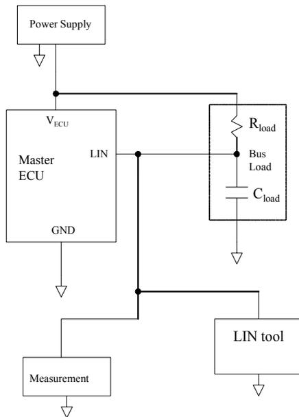
FIGURE 1—DETECTION OF ERRORS BY MASTER TEST SETUP
