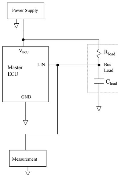
FIGURE 10—MASTER NODE BIT TIME MEASUREMENT TEST SETUP
