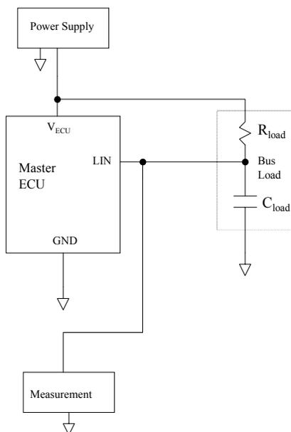
FIGURE 19—MASTER NODE  $T_{r-d \max}$  AND  $T_{d-r \max}$  MEASUREMENT TEST SETUP
