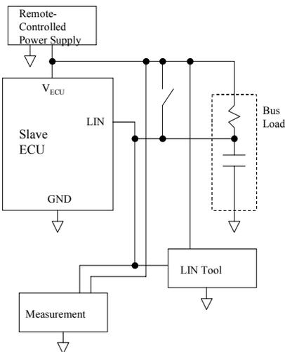
FIGURE 29—BUS WIRING SHORT TO BATTERY WITH TxD/RxD NOT ACCESSIBLE TEST SETUP
