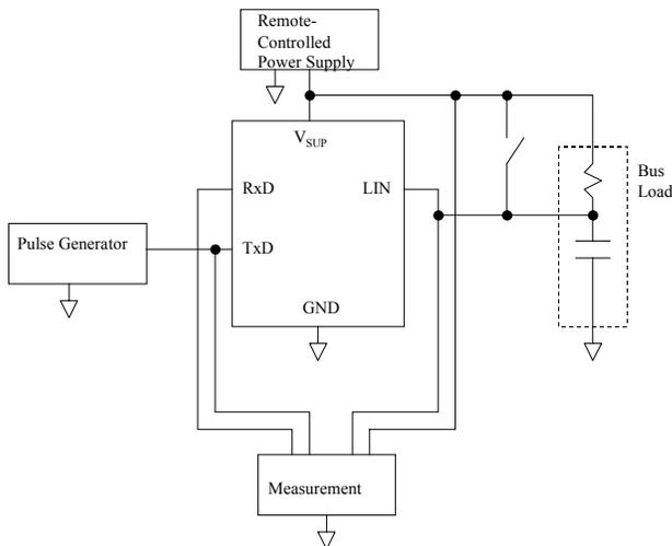
FIGURE 28—BUS WIRING SHORT TO BATTERY WITH TxD/RxD ACCESSIBLE TEST SETUP
