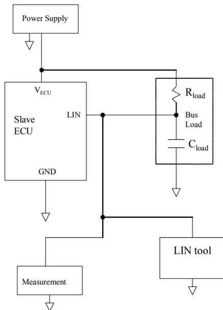
FIGURE 21—SLAVE NODE  $T_{r-d \max}$  AND  $T_{d-r \max}$  MEASUREMENT TEST SETUP
