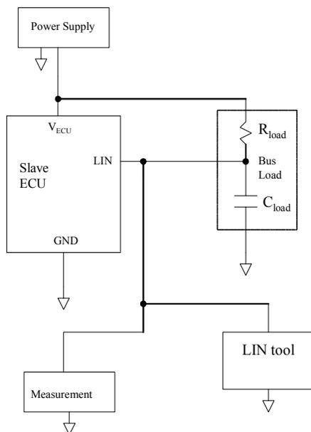
FIGURE 11—SLAVE NODE BIT TIME MEASUREMENT TEST SETUP
