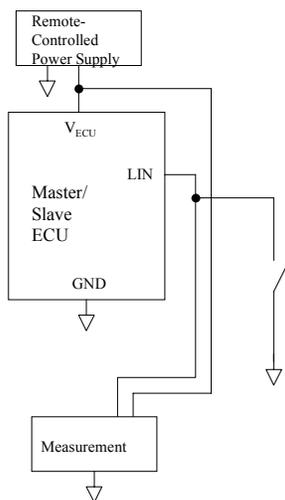
**FIGURE 27—BUS WIRING SHORT TO GROUND TEST SETUP**
