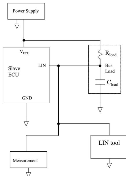
FIGURE 8—SLAVE MESSAGE ID ASSIGNMENT TEST SETUP
